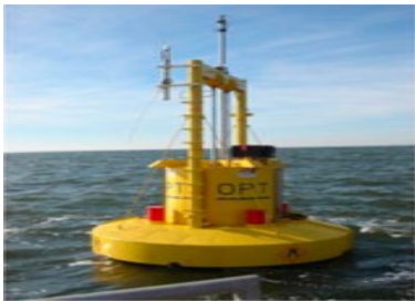
Figure 7. OPT’s Powerbuoy is undergoing development testing at Kaneohe, Oahu. It is one of several wave energy technologies being deployed in Hawaiian waters.
